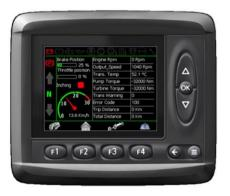
A reliable color display shows the lifting weight / lifting height / main pressure / engine status / oil level / error codes etc. all important information.
