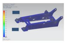
FEM analysis supported design provides high strength of chassis and mast, making whole truck stable and robust.
